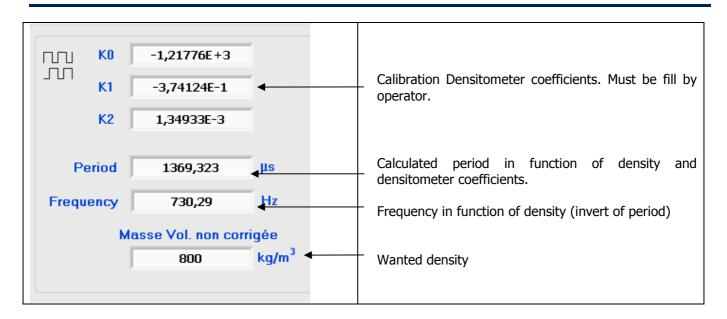
Pressure and temperature measurements can be affected to densitometer configuration for vibrating tube mechanical correction.
