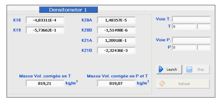
K18 and K19 correction factors are used for calculation and display of density at densitometer actual temperature.
