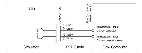
Simulated temperature is function of ohm resistor value. Resistors selected by rotary switches position 1 to 6 have following typical values: 95, 100, 102, 107, 113 et 118 Ohm. Temperature values are obtained by using ISO 60751 standard ohm / °F or °C conversion.
