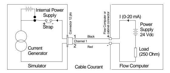
In case of current loop power supply by simulator, wiring is the following:
