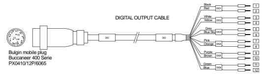
Wiring to flow computer is the following:
