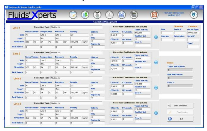
It shows four independents metering lines with volume, temperature, pressure and density measurement.
