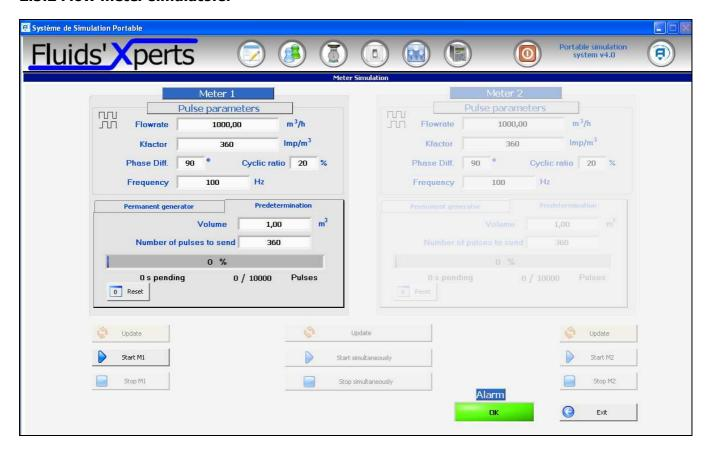
Volume or mass flow meters simulator is built around two pulse generators. These generators have two out of phase pulse outputs with frequency, electric phase, cyclic ratio and preset adjustable parameters.
