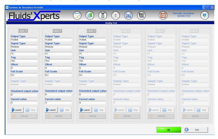
Analog outputs simulator integrates six similar and independent 0 or 4-20 mA generators.
