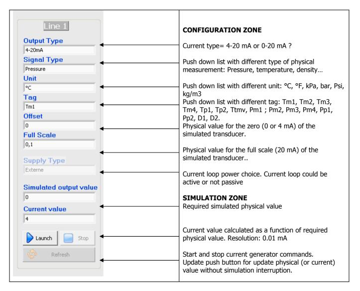
Current loop power supply: current loop could be active or passive.
