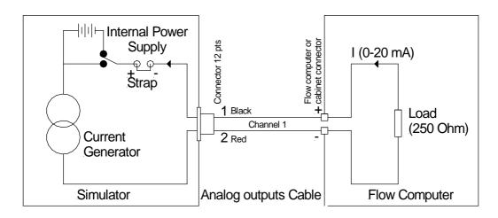
Before to choose this wiring, be sure than any voltage is delivered by flow computer on transmitter connection.
