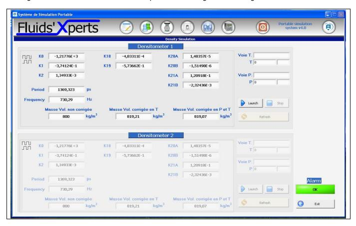
Densitometer simulator is built around two adjustable period pulse generators.
