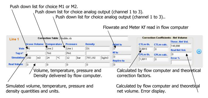
At the end of preset volume simulation, simulator read net volume and correction factors established by flow computer and calculate error with theoretical net volumes.
