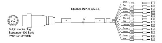
Wiring to flow computer is the following:
