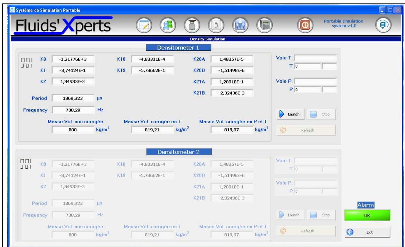
Densitometer simulator is built around one adjustable period pulse generator.
